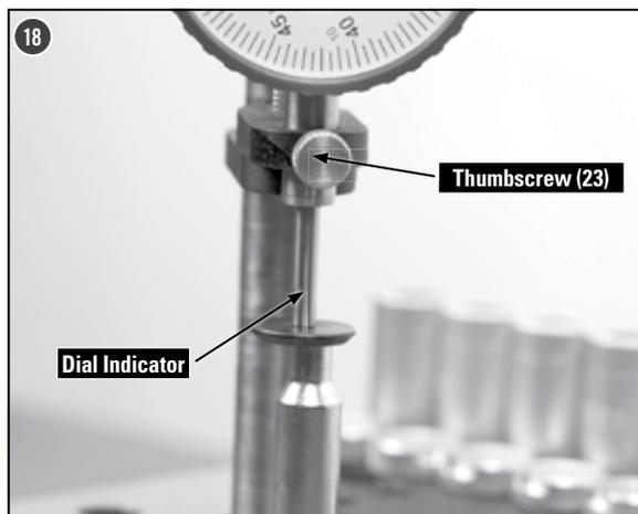
Loosen the thumbscrew on the front of Indicator Holder 2 and gently lower the dial indicator onto the mouth of the case. With approximately .100" of interference, tighten the thumbscrew.
