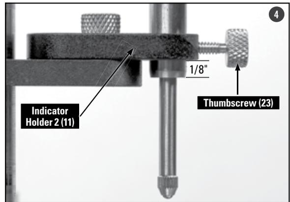
Loosen the thumbscrew (23) on the front of Indicator Holder 2 (11) and raise the dial indicator (13) in the holder until there is approximately an 1/8" from the bottom of the indicator shaft to the bottom of Indicator Holder 2. Tighten the thumbscrew.
