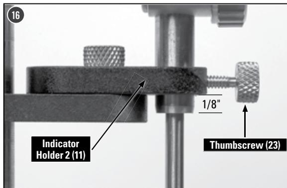
Loosen the thumbscrew (23) on the front of Indicator Holder 2 (11) and raise the dial indicator in the holder so there is approximately an 1/8" from the bottom of the indicator shaft to the bottom of Indicator Holder 2. Tighten the thumbscrew.
