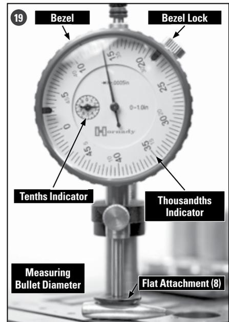
The large indicator needle on the face of the dial indicator is the thousandths indicator. Much like the tenths indicator needle, as the indicator shaft is moved upwards the thousandths indicator needle moves clockwise. Each line represents 1/2 of a thousandth (.0005), and the numbers are placed every 5 thousandths (.005). For example, the first line past 25 is .0255, the second line past is .026, the third line past is .0265, and so on.
