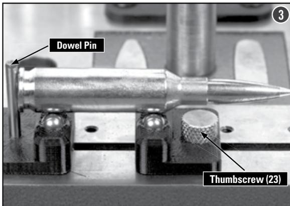
To begin, place a cartridge case or cartridge on the steel balls of the case shoulder holder (3) and case head holder (4). The case head should be pushed against the dowel pin.
