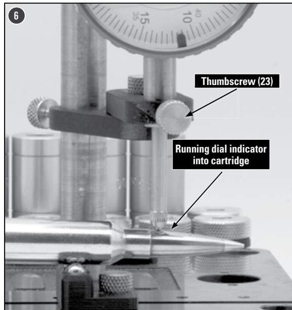
Loosen the thumbscrew on the front of Indicator Holder 2 and gently lower the dial indicator onto the neck of the case or bullet. The case/cartridge will move, but lower the indicator to roughly .100" of interference.
