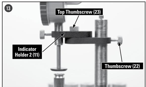
Loosen the thumbscrew on the front of indicator holder 2 and gently lower the dial indicator onto the base of the case. With approximately .100" of interference, tighten the thumbscrew.
