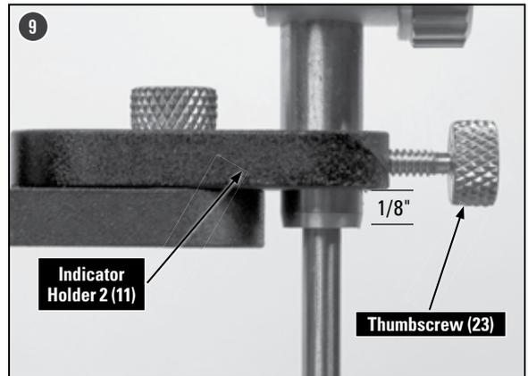
Place a bullet or cartridge in the ogive comparator. Loosen the thumbscrew (22) on the back of the dial indicator assembly and position the entire assembly to the Ogive Comparator Station so that the flat attachment is about 1/8-inch above the base of the bullet or cartridge. Tighten the thumbscrew.
