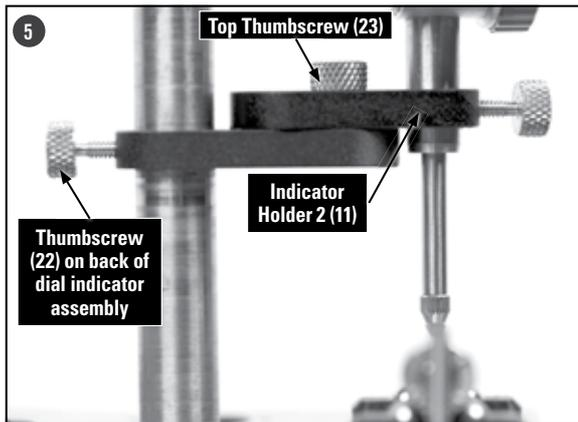
Loosen the thumbscrew (22) on the back of the dial indicator assembly. Rotate the entire assembly toward the concentricity station and adjust it so that the ball tip is about 1/8" above the bullet or case mouth. Tighten the thumbscrew.
