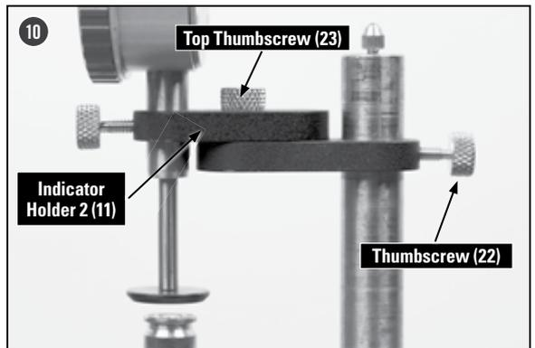
Loosen the thumbscrew on the front of Indicator Holder 2 and gently lower the dial indicator onto the base of the bullet, or cartridge if comparing base to ogive of loaded ammo. With approximately .100" of interference, tighten the thumbscrew.
