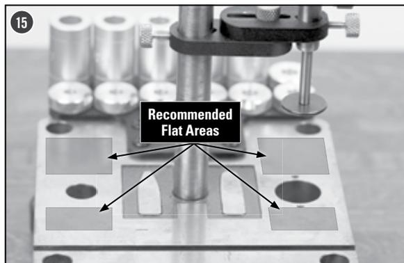
Pick a flat area on top of the Precision Measurement Station Base (1).
