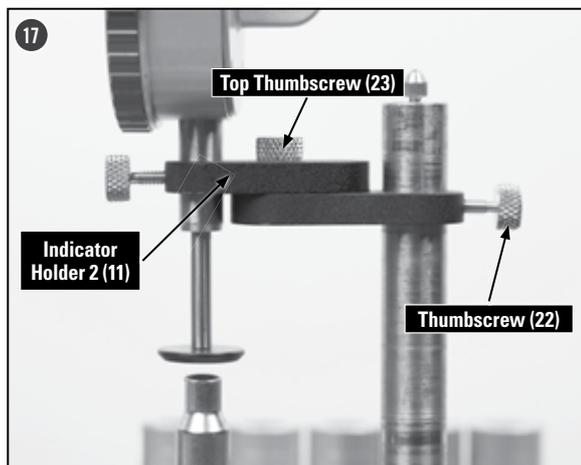
Place a case on the chosen flat section of the Precision Measurement Station Base. Loosen the thumbscrew (22) on the back of the dial indicator assembly and position the indicator so that the flat attachment is about an 1/8" above the case. Tighten the thumbscrew.
