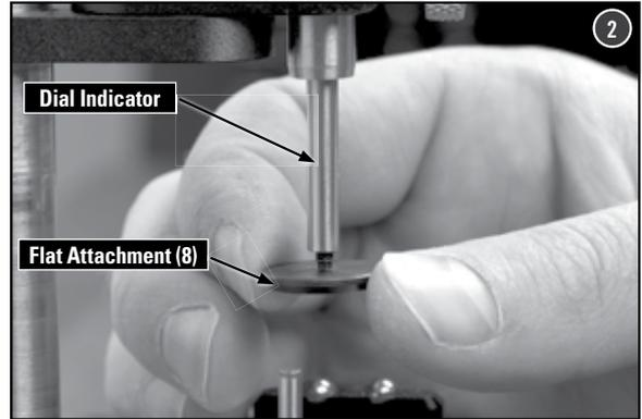
Remove the flat attachment (8) from the storage location on the top of the Indicator Shaft (2).
