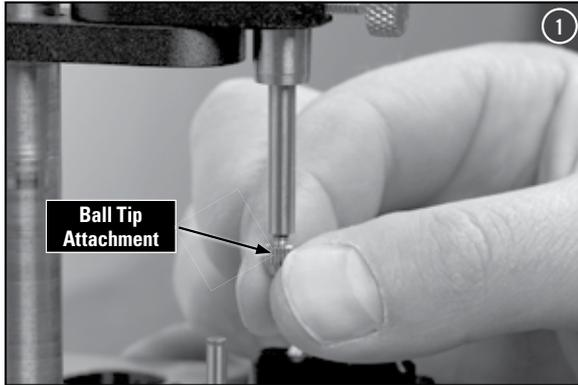
Remove the ball tip by grasping the knurled portion firmly between your fingers and turning counterclockwise. The first removal may be difficult, but **DO NOT** use pliers or any other mechanical means to remove the ball tip. This could damage the dial indicator and the tip.
