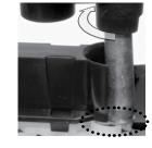
assembly into the base casting hole, and adjust the top nut so that the bottom of the feed plate assembly rests on top of the coin. Tighten the top nut so that the feed plate assembly clears the frame using a 7/16" wrench.
