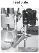
Re-attach the spring to the case actuator and test operation on a few cases. If the cases drop too soon, they may rest on top of feed fingers. Rotate the feed tube support farther away (clockwise) from the press to delay the dropping. Because of the wide range of diameters and rim configurations, you will have to fine tune this position to provide reliable feeding.
